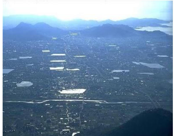
A plain in Kagawa with various small water impounding reservoirs, each of which are systematically located and connected with one another
